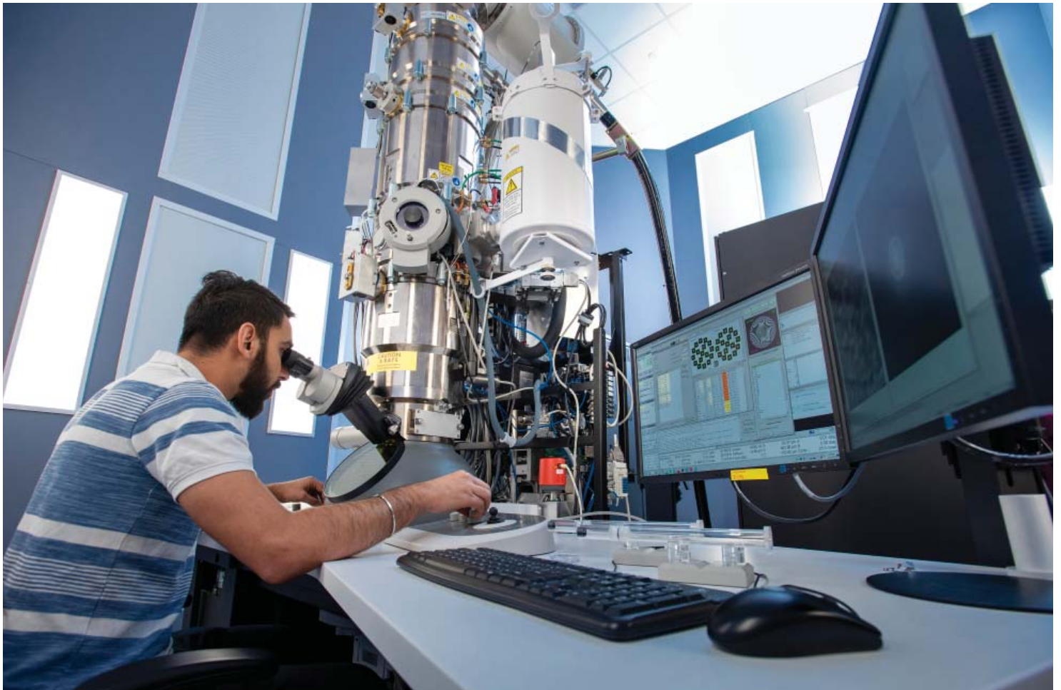
MSE Ph.D. student Sarshad Rommel works at the Titan Themis S/TEM (scanning/transmission electron microscope)
