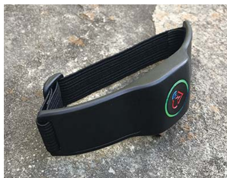
Prototype of Mobile Sense Technologies' wearable device to detect arrhythmias. (Photo courtesy of Mobile Sense Technologies)
